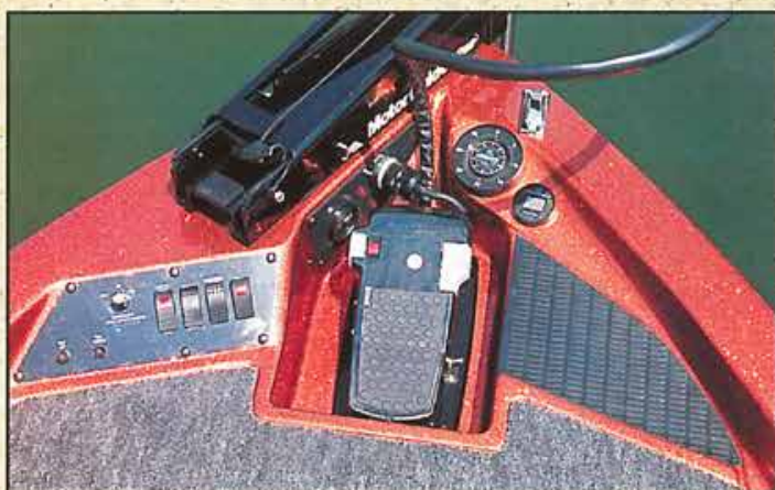
Front Bow Layout on the Pantera Classic and Pantera II, the Eyra is Similar With an Extended Recessed Area to Right of Trolling Motor Basin for Bow Mounted Graphs.
