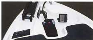
A Wider Bow With Recessed Trolling Motor Pedal Mount and Graph Area.
