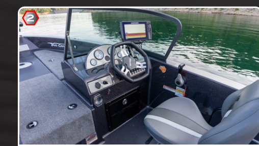
2 All-fiberglass dash with under-console storage with removable, lockable doors.
